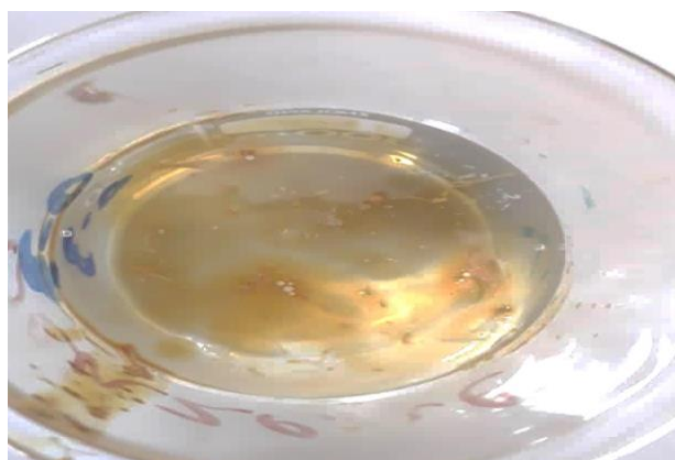
Figure 1. Process of crude oil removal from seawater using Nano magnetite (a) mixture of crude oil with CFA-CFO in seawater, (b) attraction of crude oil with CFA-CFO in seawater by magnetite.
